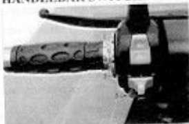
1. Dimmer switch 2. Turn switch 3. Horn switch
