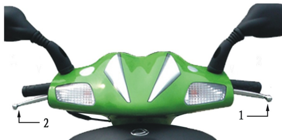
1. Rear brake lever 2. Front brake lever
